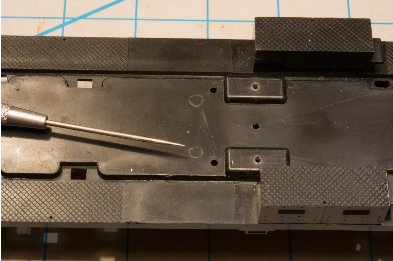
Figure 6.2. Use scribe marks to locate new drilled holes. (RS-3 model shown)
