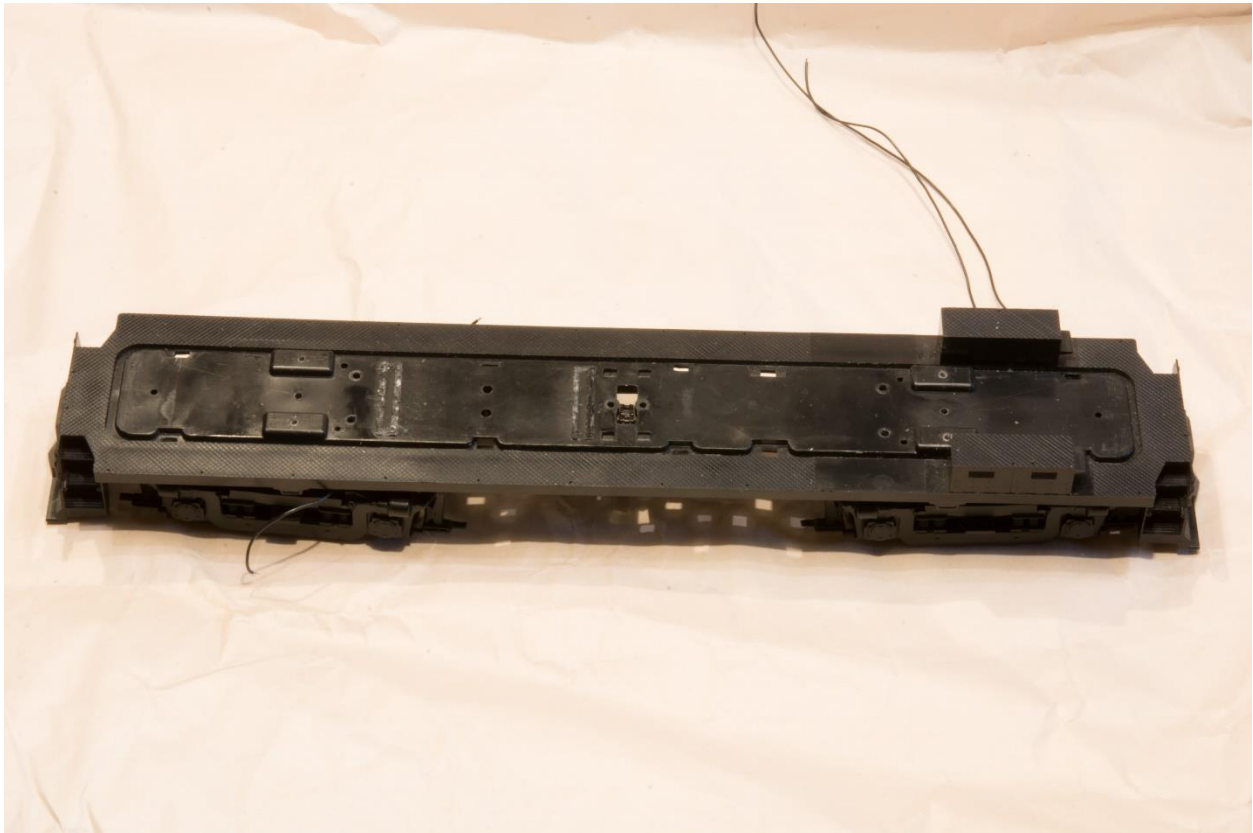
Figure 5.1. Bare frame with motor mounts removed.
