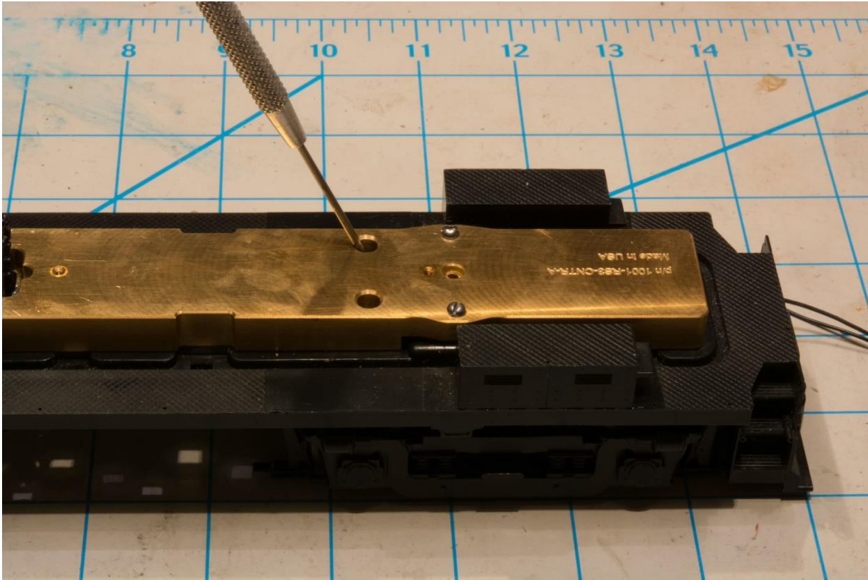
Figure 6.1. Use scribe to mark new wire pickup hole locations.
